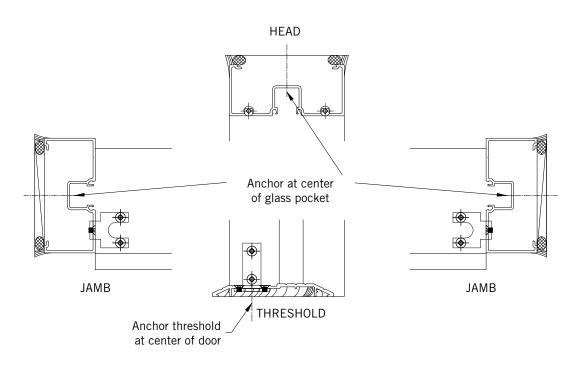
Figure L-2 Offset Fasteners
