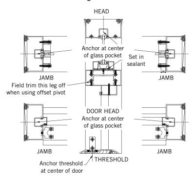
**Figure Z-2**Offset Fasteners
