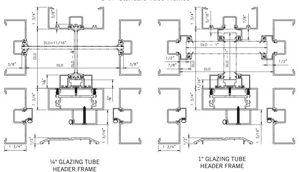
Figure F-2 2" Standard Tube Frames
