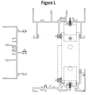
Frame weather stripping at operable panel side
