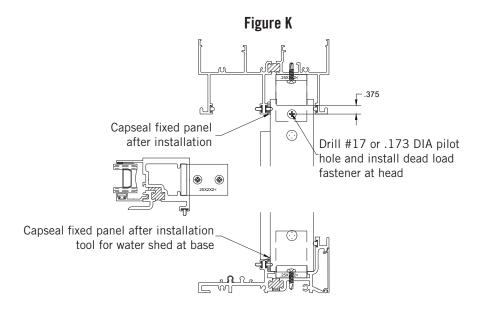
Install panel clips and capseal perimeter of fixed panel
